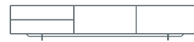
Cabinet with right deep drawers and left lockable drawers 1CE6053: L 200 D 65 H 54,5 1CE6054: L 298,5 D 65 H 54,5 1CE6057: L 200 D 65 H 54,5 (with finishing back) 1CE6058: L 298,5 D 65 H 54,5 (with finishing back)
